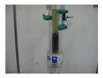
Fig. 5 Picture of the inside column where DME was circulated upward from the bottom. (The dark-colored lower half portion is blue-green algae and the light green liquid in the upper half is DME, including extracted "Green Crude Oil")
