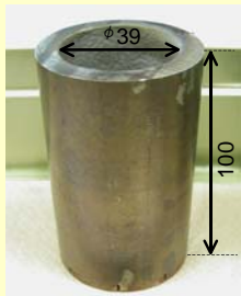
Pipe with corrosion product film including cobalt-60
