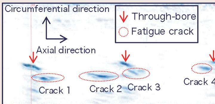
(b) Example of the detection of cracks in an open rack vaporizer
