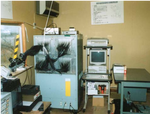
ALPS and observed results of upward leader (ALPS: Automatic Lightning-discharge Progressing-feature observation System)
