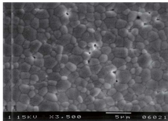
**Fig.4** Scanning electron microscopy (SEM) micrograph of CGO electrolyte on the porous anode in IT-SOFCs
