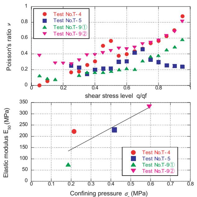
**Fig.4** Mechanical properties of the site
