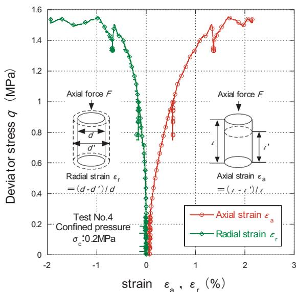
**Fig.3** Relationship between stress and strain
