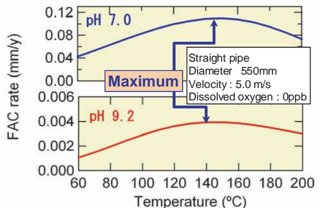
**Fig.6** Effect of temperature on the FAC rate
