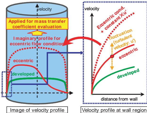
**Fig.1** Concept of mass transfer model in eccentric flow
