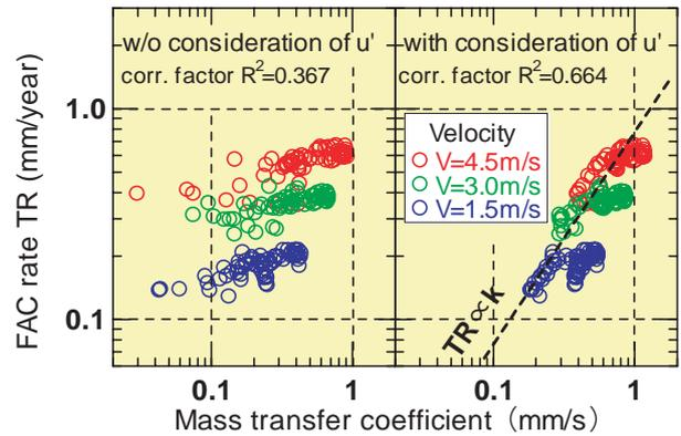
**Fig.2** Correlation of FAC rate and mass transfer coefficient
