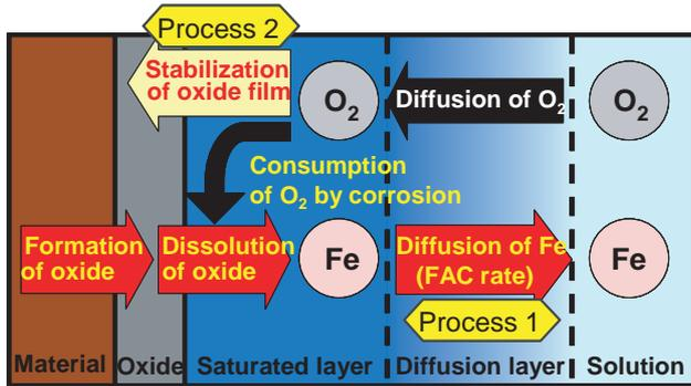
**Fig.3** Schematic of FAC model
