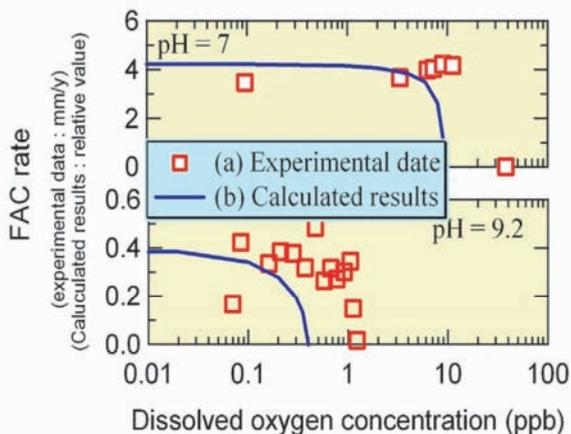
**Fig.5** Effect of dissolved oxygen on the FAC rate
