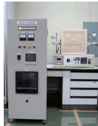
Photo 2 Vacuum furnace (right) and temperature monitoring system for vacuum furnace (left)
