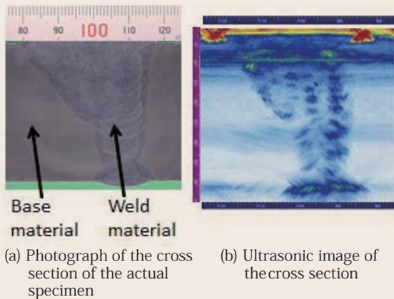
Fig. 1: Estimation of the shape of weld metal
