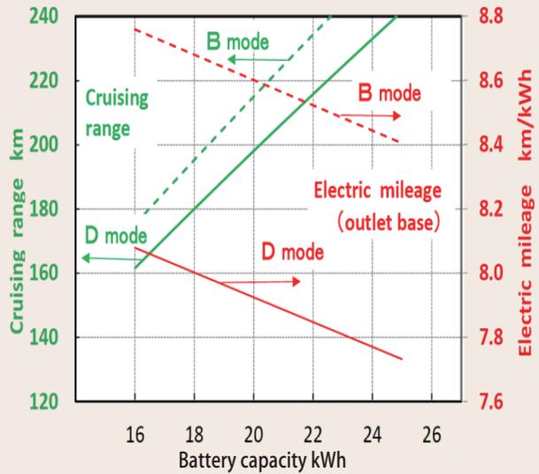
Fig. 2: Evaluation of driving mileage against the battery capacity mounted on EVs
