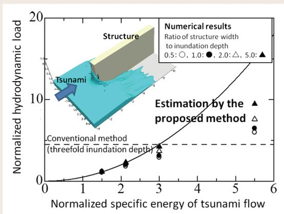
Fig. 1: Comparison between tsunami hydrodynamic loads predicted using the proposed method and those obtained by three-dimensional numerical simulations
