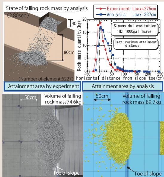
Fig. 2: Verification of evaluation method of rock mass attainment area due to slope collapse by numerical simulation of shaking table test
