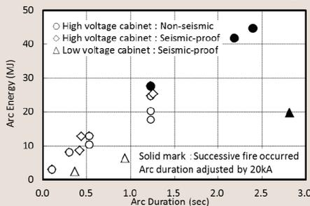
Fig. 3: Arcing energy measured in HEAF tests using low-voltage electric cabinets and the limitations of fire occurrence
