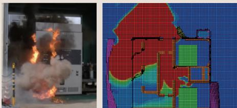
[Examples of HEAF test with low voltage cabinet and simulation for zone of influence]
