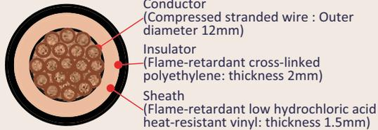
[Cross section of inflammable low voltage power cable]
