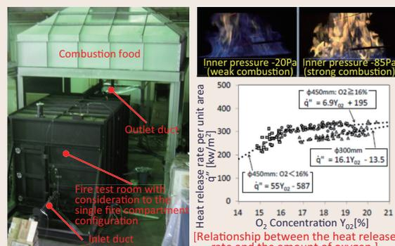
Fig. 4: Identification of heat release rate in a compartment under ventilation conditions
