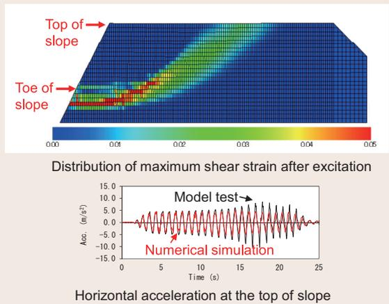
Fig. 1: Numerical simulation of dynamic centrifugal model test of slope (upper part: distribution of strain, lower part: comparison with the experiment of response acceleration)
