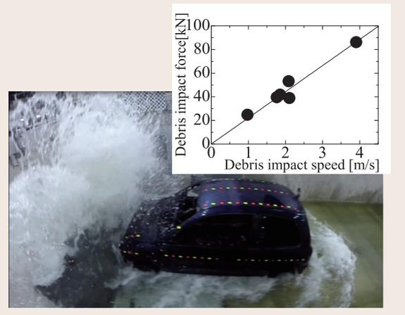
Fig. 4: Evaluation of tsunami-debris impact force
