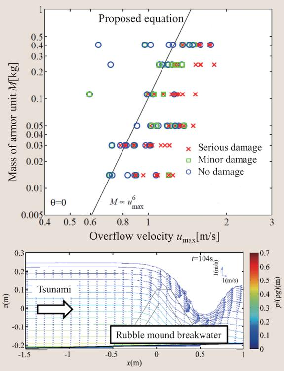
Fig. 2: Stability assessment of rubble mound breakwater
