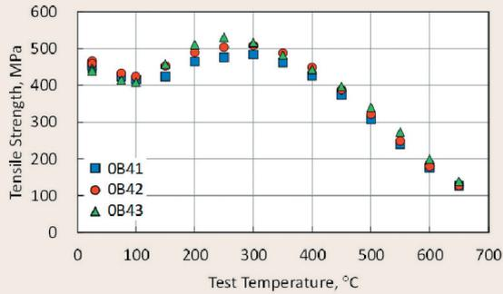
Fig. 1: Effect of test temperature on tensile strength for SN steel (SN400)
