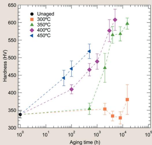
Fig. 3: Relationship between hardness of ferrite phase and aging condition
