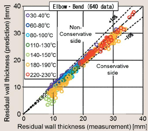
Fig. 2: Prediction accuracy for residual wall thickness of 4 PWRs' elbows by FALSET
