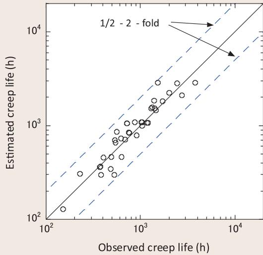
**Fig. 1: Estimated results for creep life of 9Cr steel welded joint**
